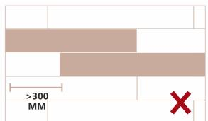
The longest side should be staggered no more than 300mm when laid in running bond.
